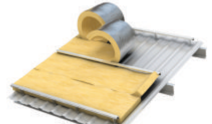
Fig ii: Bulk insulation to the required depth can then be installed over the liner sheet or existing roof. Care needs to be taken that the bulk insulation is packed tightly to avoid thermal bridging. It is recommended practice to stagger the joints of the insulation when more than one layer is installed. It is imperative that a vapour barrier be installed in high condensation regions.
