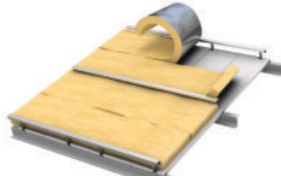
Fig b: Bulk insulation to the required depth can then be installed over the installed rigid boards. Care needs to be taken that the bulk insulation is packed tightly to avoid thermal bridging. It is recommended practice to stagger the joints of the insulation when more than one layer is installed. It is imperative that a vapour barrier be installed in high condensation regions.
