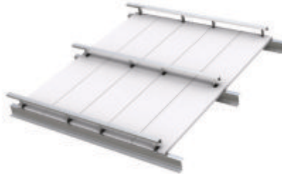
Fig a: In the above configuration rigid insulation boards are installed over purlin. The rigid insulation boards need to be secured to the purlins by means of self drilling fixings with a 45mm diameter fender washers to alleviate movement in negative pressure environments. The Ashgrid Spacer System is installed by recessing the brackets through the rigid insulation boards and securing to the purlins. This creates a defined roof cavity to accommodate the insulation.
